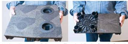
Interchangeable carpet tiles self-adhere to a set of four pedestals. This allows flex, so they float on the floor without laser leveling. Universal outlet ports for power, data, AV or pass-thru may be located in any of the pedestals. Pedestals are 3" high, providing a generous cable way capacity. Weight capacity tested to 40,000 lbs for each pedestal. 20 US tons.
