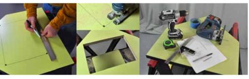
iPad flipIT Kit<sup>®</sup> installs in any table top using basic carpentry skills. Power tools are required to make the cutout in the table top. iPad flipIT<sup>®</sup> may also be specified to be factory installed in most SMARTdesks classroom furniture. Order the iPad flipIT<sup>®</sup> online—only at www.smartdesks.com.
